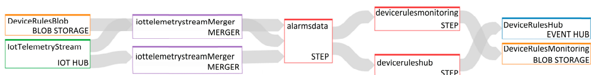
Figure 4. Job diagram for device telemetry stream.
